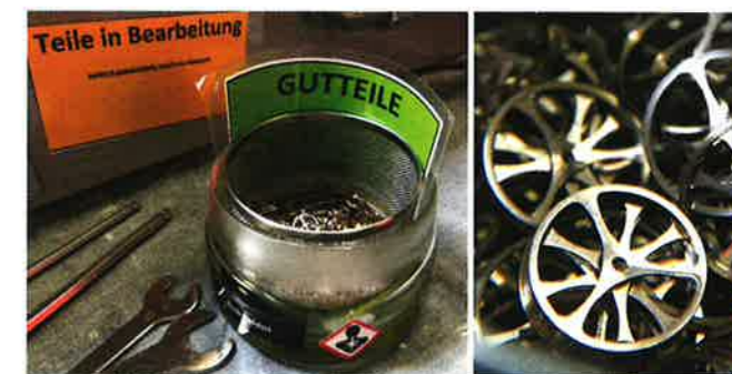
Figures 2A and B. Cupro-nickel balances, fresh off the sliding-head lathe.
