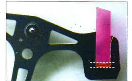
Figure 8. This gap is gauged as large, medium or small, and pallets with a suitable gap are chosen when controlling the amplitude of a new watch.
