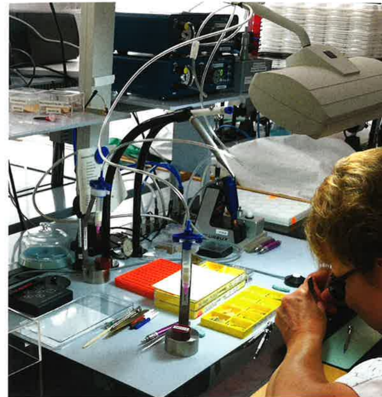
Figures 7A. At this assembly station, the lady is surrounded by aids to her work. Micro-dose dispensers ensure predictable and clean oiling. Automatic pneumatic screwdrivers start rotating when they are pressed down.
